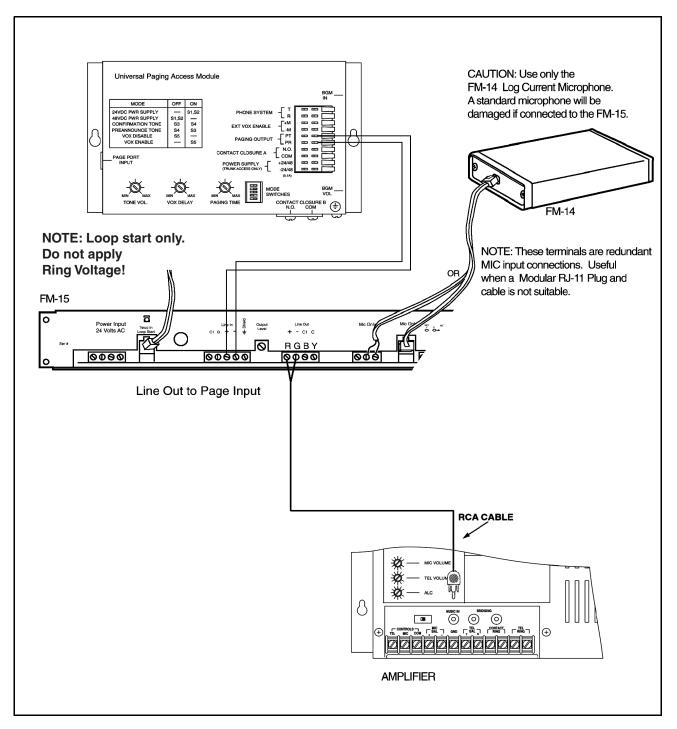
Figure 3-3. FM-15 ALC Connection to a LUUPAM Universal Paging Access Module
